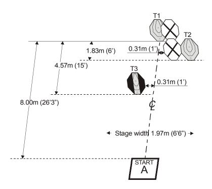
**SETUP NOTES:** Set paper targets to 1.52m (5 feet) to the top of targets. Hard cover on T3 is even with edges of the A zone. Penalty targets are placed on T1 and T2 so that they are the same height and that the perforation line of the A zone is overlapping by the perforation of the penalty targets border of the penalty target. Area A is 1m(3'3") by 1m(3'3").
